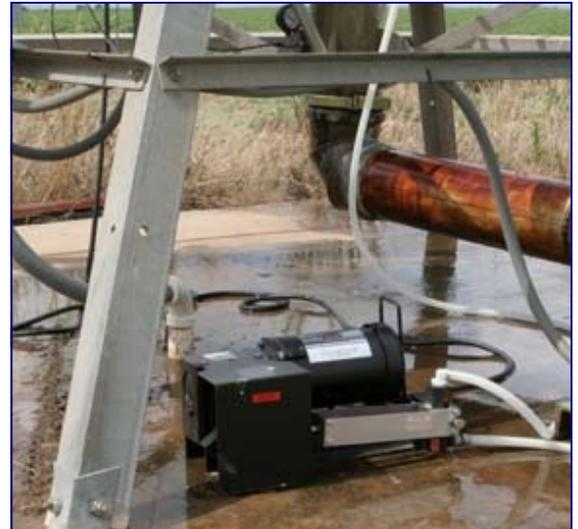
pumps are self-priming and should clear itself of air in a few minutes. If not, check the stroke length and make sure it is at full stroke, this will enable any particulates to be flushed through the pump.
