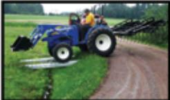
**Ditch bridges 5 - 20 Ton rated capacity. Designed to cross ditches for cranberry farmers.**
