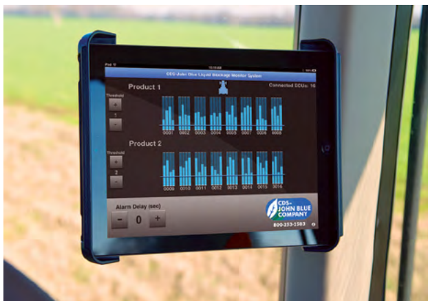
Electronic Liquid Blockage Monitor System (LBMS)
