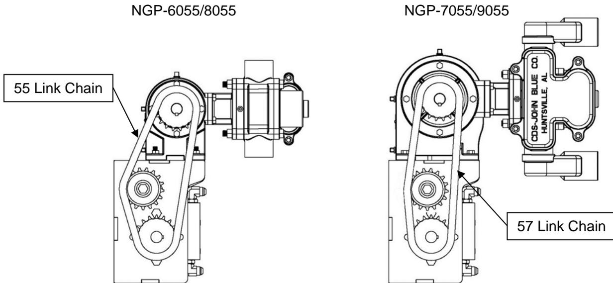
F.) Slide the idler sprocket over in the slot to tighten the chain, and then tighten the nut and jam nut to lock in place.
