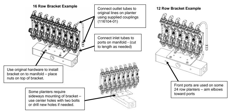
4. Attach mounting bracket onto manifold using the original bolts and nuts. Note: feed the bolts from the bottom of the bracket and place the nuts on top. *Do not over tighten!* (5 ft-lbs max)
