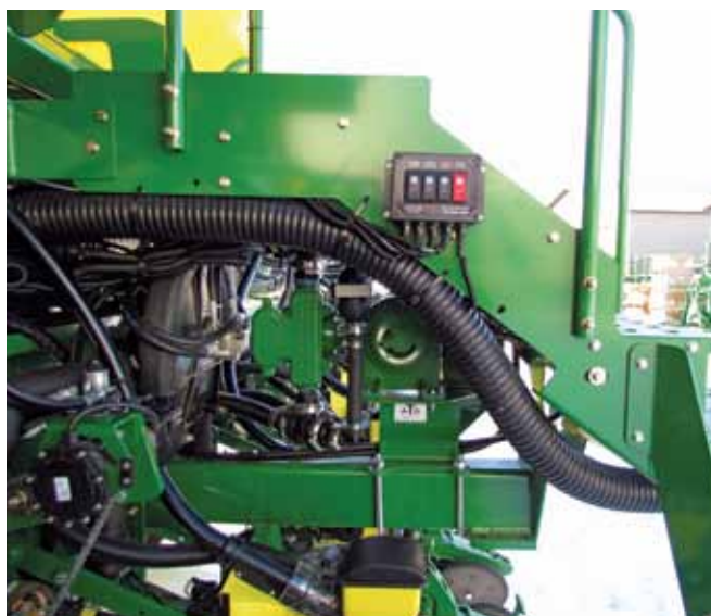
This electric bypass harness system from Total Ag Industries allows for quick troubleshooting on the planter. Installation includes two, three or four buttons on the rear of the planter depending on its size. A press of the button engages the system for lubrication, priming and winterizing.
