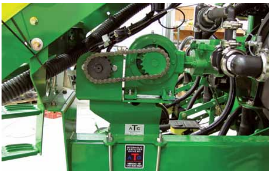
Variable rate hydraulic drive fertilizer systems can provide precise control and accurate application in the field. Total Ag Industries builds the systems with CDS-John Blue components and can install it on most new and used tillage and planting equipment.
