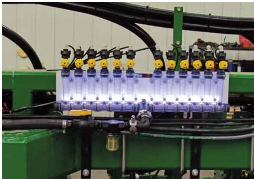
Working with dealers and farmers, Total Ag Industries custom-builds fertilizer systems and installs them on new and used planters. Above: Back-lit sight-glass flow monitor systems give the tractor operator visual confirmation the fertilizer system is working properly.
